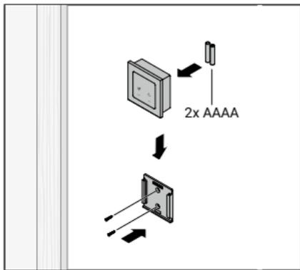
1. At the installation location of the control unit, mount the wall bracket at standard height to the wall using the screws and dowels supplied, so that the labelling TOP points to the top.
