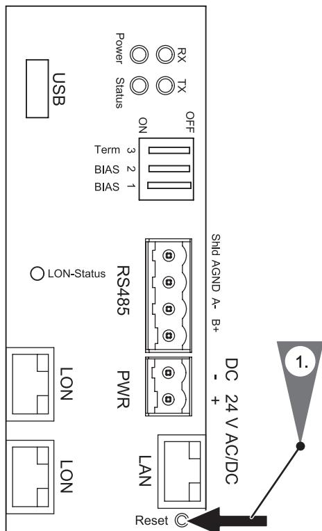
1. Press the reset button with the tool supplied or another thin object for 1 to 2 sec.
