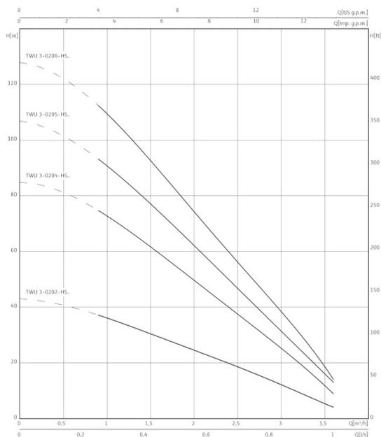
1~230 V, 50 Hz,  $\rho = 1 \text{ kg/dm}^3$ ,  $\nu = 1 \times 10^{-6} \text{ m}^2/\text{s}$ , ISO 9906 Anhang A,  $\eta =$  Pumpenwirkungsgrad
