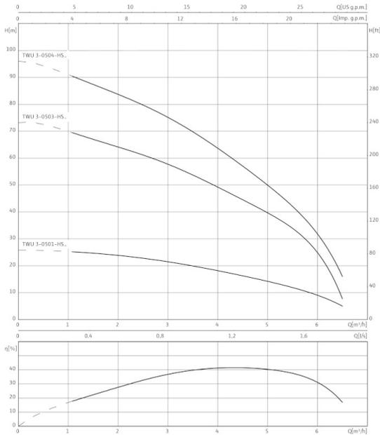
1~230 V, 50 Hz,  $\rho = 1 \text{ kg/dm}^3$ ,  $v = 1 \times 10^{-6} \text{ m}^2/\text{s}$ , ISO 9906 Anhang A,  $\eta =$  Pumpenwirkungsgrad
