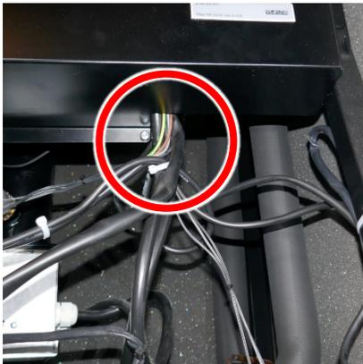
33. Fühler an PIL-Leiterplatte anschließen: [18] → T6, [19] → T8, [20] → T9, [21] → T10, [22] → T11, [24] an LP.
