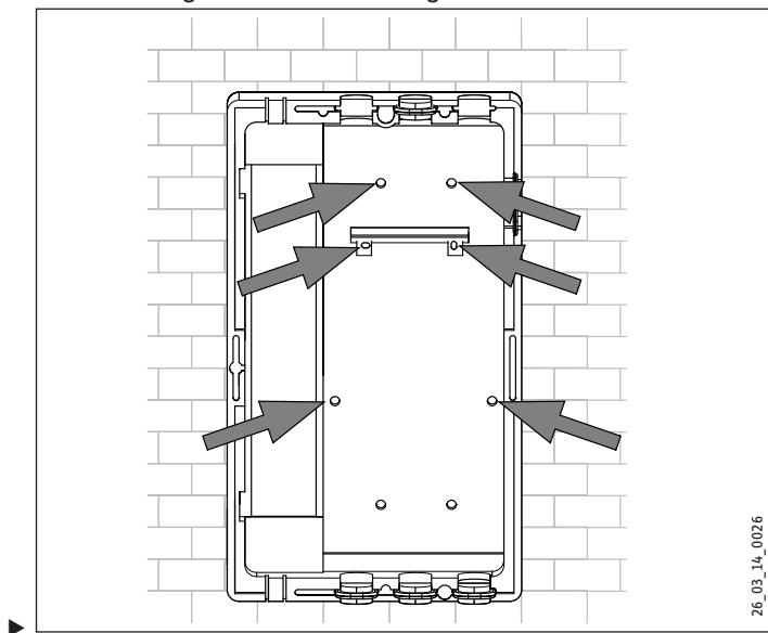
Drill the holes and insert rawl plugs.
