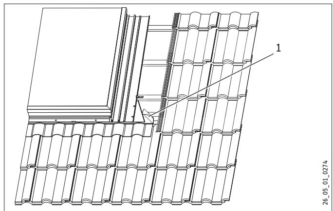
1 Piece of lead flashing
