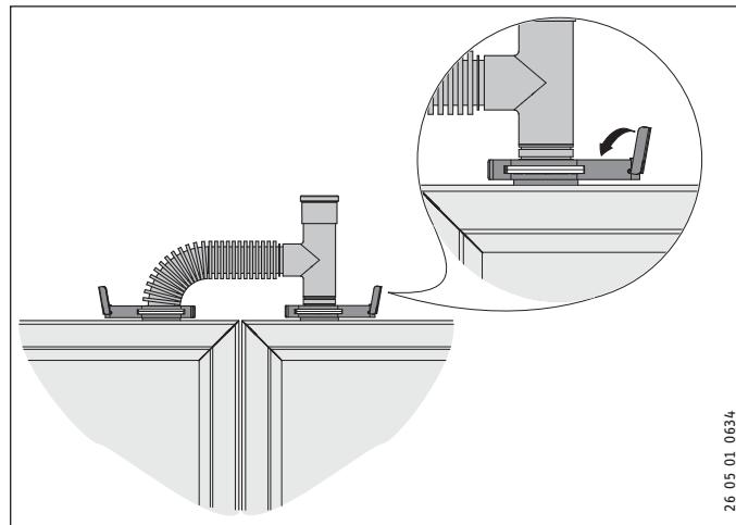
Plug-in connection SV-I is used to connect the collectors (see "Required accessories").
