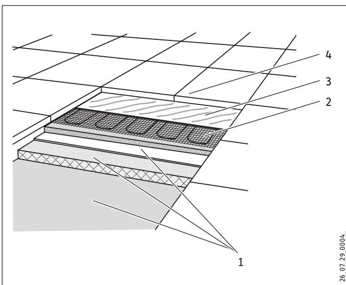
1 Substrate with thermal insulation
