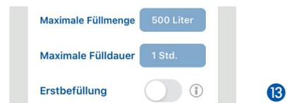
13 Start the "Erstbefüllung" (initial filling) by pulling the slider to the right.
