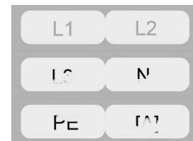
Fig. 3: Print-out faint and incomplete
