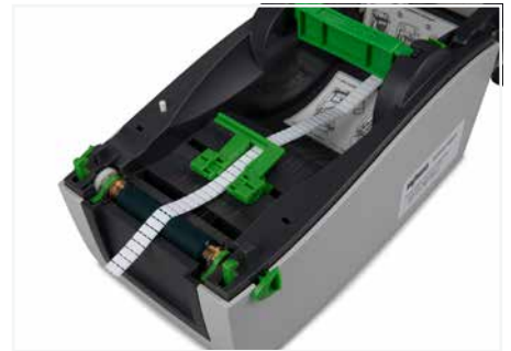
Loosely fit guide rails to the material.
