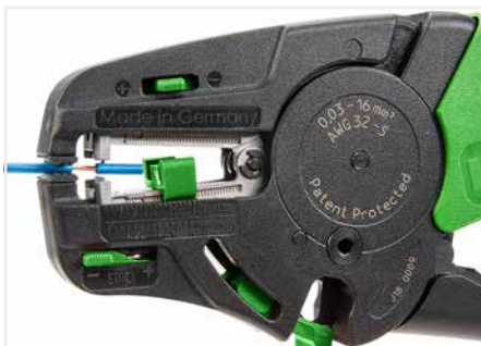
Partially stripping a conductor.
