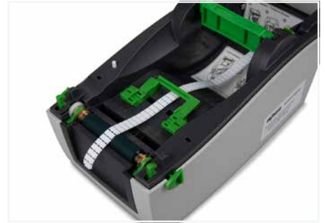
Guide the marker strip over the roller.
