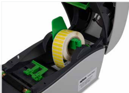
Loosen the center bar, loosen the wing and place material on the bar.
