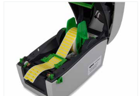
Secure the second wing on the center bar, resecure the bar in the housing and loosely attach guide rails to the material.
