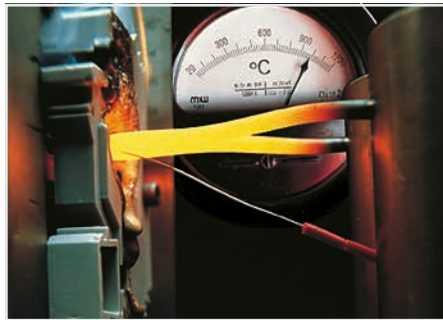
Glow-Wire Test per IEC/EN 60998-1, IEC/EN 60695-2-11
