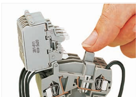
Commoning Distributing current to several fuse-protected circuits via insulated push-in type jumpers.
