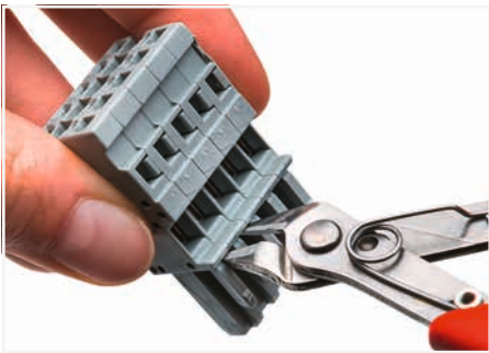
Coding a female plug by removing coding finger(s) via cutting tool. Do not remove the first and last coding fingers or use an additional locking lever.
